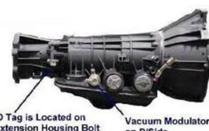
ID Tag is Located on Extension Housing Bolt
